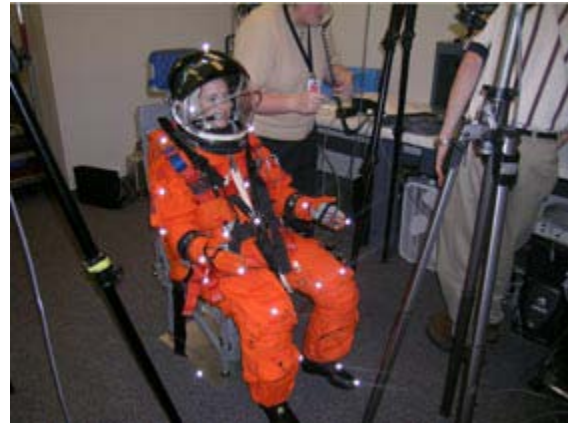
Figure 2: Advanced Crew Escape Suit (ACES) Seated Motion Analysis
