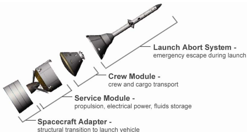
Figure 1: Components of the Orion spacecraft (NASA concept)
