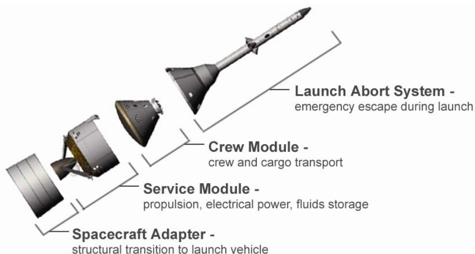
Figure 1: Components of the Orion spacecraft (NASA concept)
