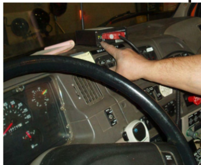
Display/alarms activated by truck driver
