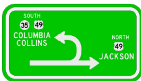
Figure 23: Recommended Signage at the Left Turn (J-Turn) Intersection of an RCI
